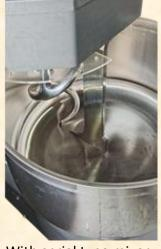
. With sprial type mixer,. With static vertical dough scraper,
