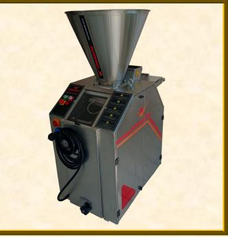
This is a machine ,that divides the dough placed in its hopper into desired weights.
