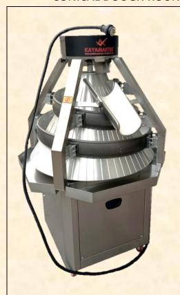
The dough rounder gives a round shape to the dough thanks to an aluminum cone with vertical channels, rotating on its own axis, and motionless (but adjustable in width) aluminum arms circulating around it in a spiral.
