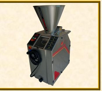
This is a machine ,that divides the dough placed in its hopper into desired weights.
